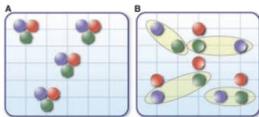
**Fig. 1.** Three-species fermionic atoms (red, green, and blue spheres) in an optical lattice can form two distinct phases when the interactions between the atoms are tuned. In the first case of strong attractive interactions between the atoms, they join as “trions” (A), whereas in the second case of weaker interactions, a color superfluid is formed (B), in which atoms pair up between only two species. The two phases have strong analogies to the baryonic phase (A) and the color
