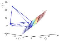
• Polytope for N = 10 and J = (0, 0, 0). States that are detected by the KCL criterion are below the plane. The plane contains two of the three  $A_k$  points.
