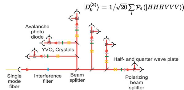
input state from the photon source is split up into spacial modes
