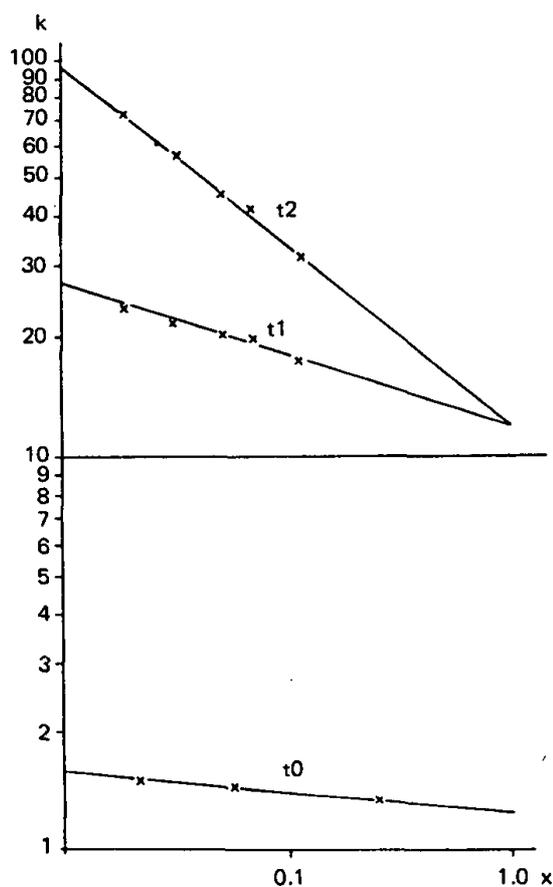
FIG.2. Plot of  $\log k$  versus  $\log x$  for L-tyrosine (t0), 3-iodo-L-tyrosine (t1) and 3,5-diiodotyrosine (t2) (eluent: water/ethanol, pH 4).
