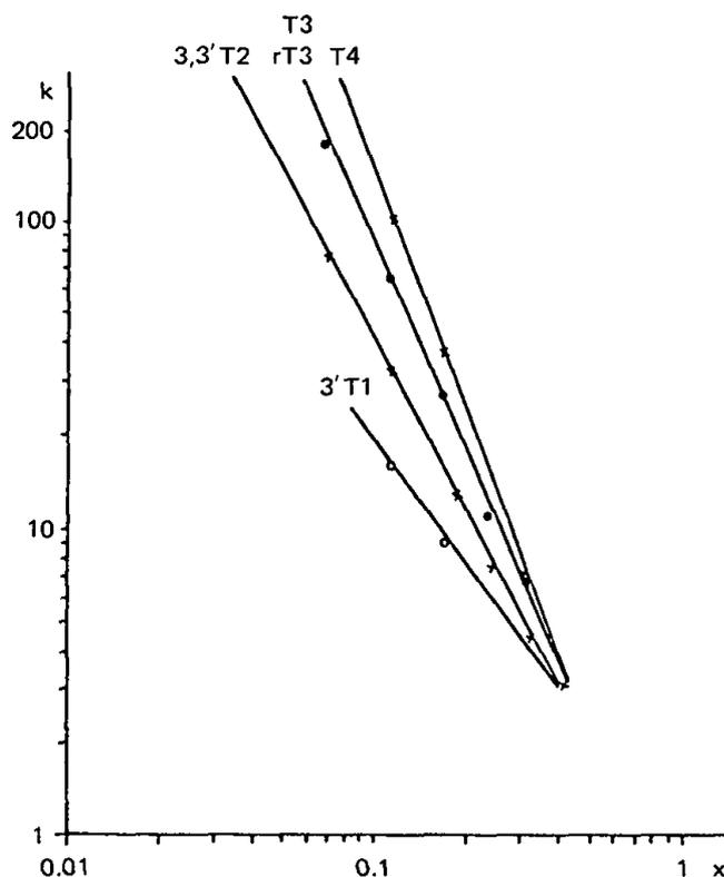
FIG. 3. Plot of  $\log k$  versus  $\log x$  for iodothyronines (eluent: water/ethanol, pH 4).
