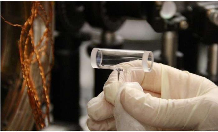
Picture of the glass cell that where the rubidium metal is mixed with nitrogen gas and heated up to 450 degrees Kelvin. At that high temperature, the metal vaporizes, creating free rubidium atoms that diffuse around inside the cell. Image credit: © ICFO
