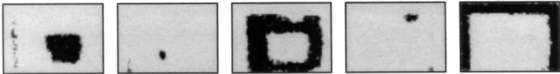
Figure 12. The depth layers found for a real scene stereo pair of two boxes with projected pattern
