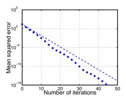
Time dependence of the error for two qubits for the deterministic method using two unitaries.
