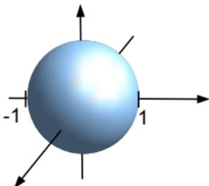
Set of physical quantum states for a single qubit. The axes correspond to  $v_l$  for  $l = x, y, z$ . Pure states correspond to points on the surface, mixed states correspond to internal points.
