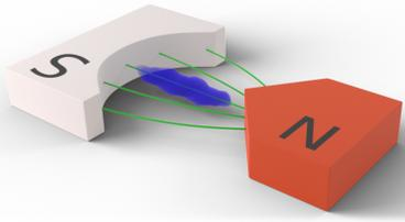
Representation of an atomic cloud in a magnetic field with a gradient term different from zero, similar to the Stern-Gerlach apparatus.
